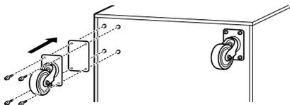
For installing the optionally available Yamaha SPW-1 wheels. To install the wheels, use these screws after removing them from the unit. Do not use the CXS once the screws are removed. This causes air leaks to occur in the enclosure, resulting in undesirable performance.
