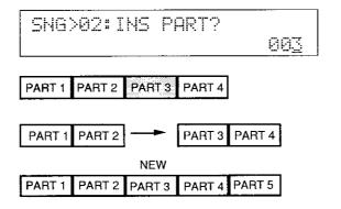
When the insert operation is executed the existing part 3 and all subsequent parts are moved up, leaving space for a new part 3 which should be recorded immediately after the insert operation is executed (while the TYPE and event parameters are flashing).
