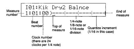
5. To enter a note, use the  $[\triangleleft]$  and  $[\triangleright]$  keys to move the cursor to the appropriate location on the measure display, then press an instrument pad.
