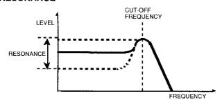
Higher resonance values produce a higher resonant peak, emphasizing a narrow band of frequencies at the filter's cutoff.
