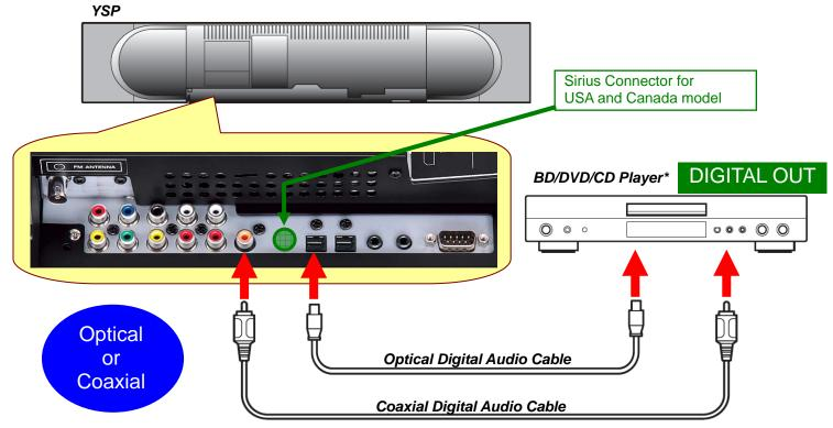
\*It is recommended to remove all other connection from the player. If the player is connected to another amplifier/receiver, make sure those components are powered off. Or else, the loud digital communication sound output during the update could cause damage to the speakers.
