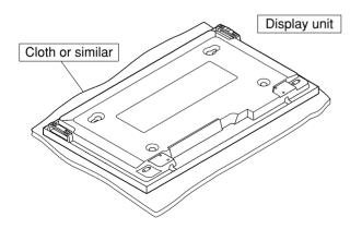
Spread a clean cloth or similar material over a level floor or base, and place the display unit on it face down.
