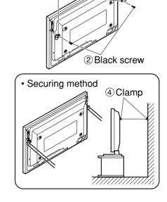
\* Use strong wire or chain which is commercially available to secure the wide plasma display to a solid area of the wall or a pillar.
