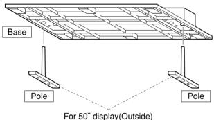
Insert the poles into the left and right holes in the underside of the base so that they fit securely as shown in the illustration above.
