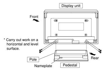
Use the assembly screws (2) (Black screw) to fasten securely.
