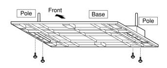
Use the assembly screws (1) to secure the poles firmly to the bottom of the base.
