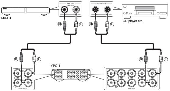
Turn off the power of the power amplifier, and then use high-quality, short audio pin cables to connect the power amplifier. You can connect up to five components that feature analog audio output jacks. Use high-quality audio pin cables for connection.
