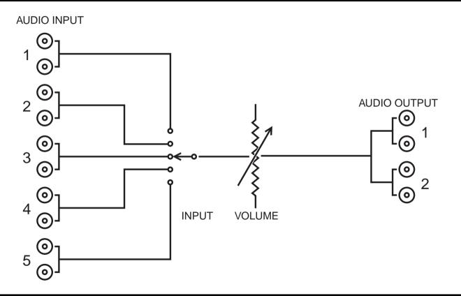
The VOLUME control features a precut brass case, gold plated multi-contact brush, and low-resistance, low-distortion carbon ink, which together provide very smooth operation and an L/R linkage error of  $\pm 1$  dB or less.
