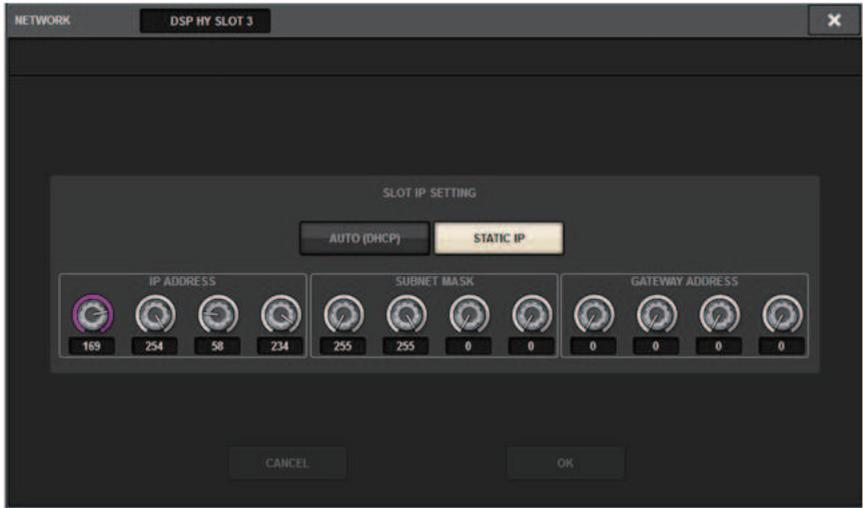
**AUTO (DHCP)...** The IP address is obtained automatically.
