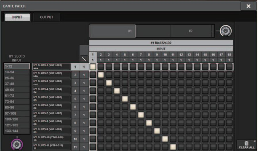
Specify the patching that will be input from the I/O rack to the Dante-enabled HY card.
