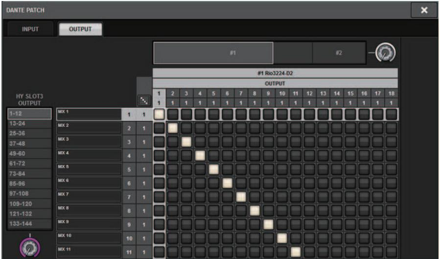
Specify the patching that will be output from the Dante-enabled HY card to the I/O rack.
