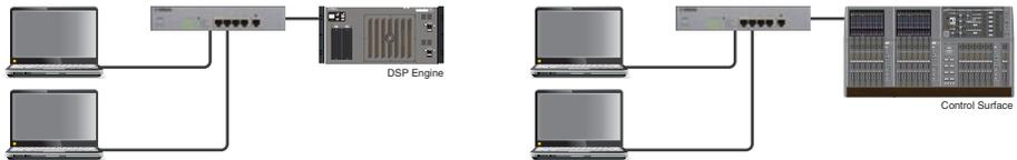
If you want to connect two computers to a DSP engine or control surface, use a switching hub to make connections.
