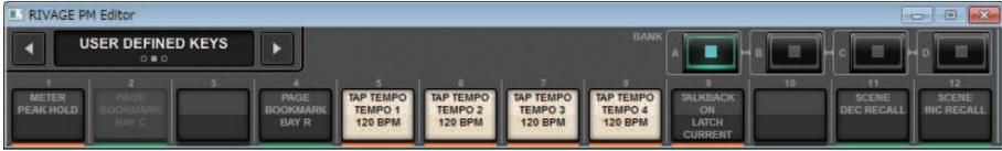
You can switch the functions assigned in the USER DEFINED KEYS screen on or off. Buttons for the functions that you cannot control in PM Editor will be grayed out.
