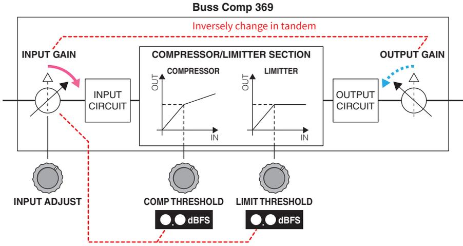
Practically, since the threshold changes, the indicated value will change in tandem. However, the internal status of the COMPRESSOR/LIMITER section will not change.
