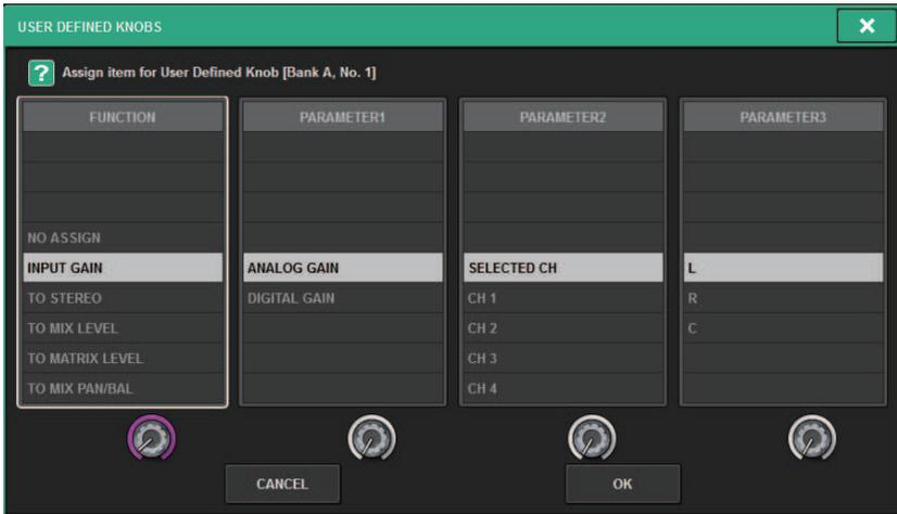
**4 Make sure that the FUNCTION field is enclosed by a frame, and then use the screen encoder on the panel to select the function that you want to assign.**
