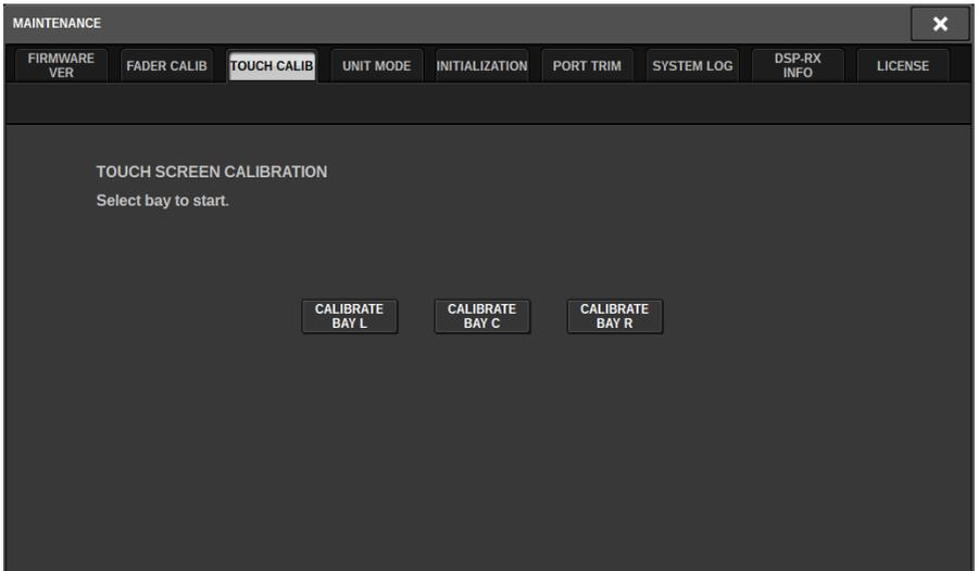
**4 Select the bay for which the touch screen panel will be adjusted, and press the button.**
