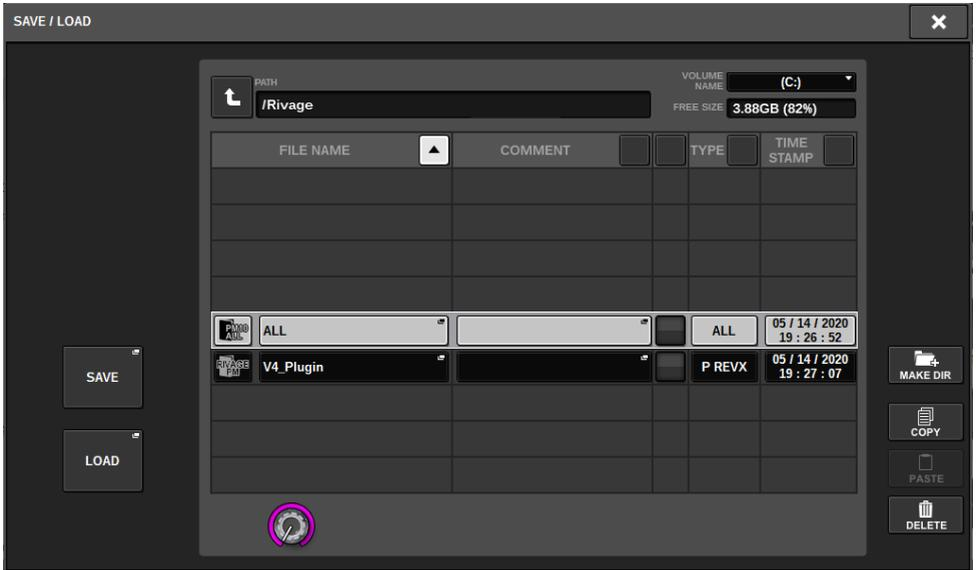
In PM Editor, you can specify a directory to/from which to save or load a file. The file format that PM Editor supports is expressed with the extension .RIVAGEPM. Internal setting files of the RIVAGE PM series will be saved.
