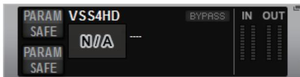
These are shown for the sake of file compatibility with the RIVAGE PM10 series, but will not perform audio processing. They can be changed to another plug-in or unmounted.
