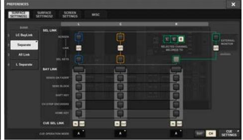
L Separate... This option is suitable for two operators. For example, operations on bay (L) will not interfere with the operations on bay (C&R).
