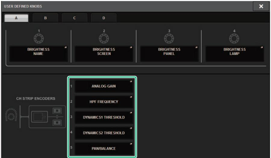
**3 Press a button in the CH STRIP ENCODERS field to open the CH STRIP ENCODERS popup window.**
