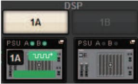
In the case of a DSP mirroring configuration, this area will display a button for switching the DSP engine between active and standby, and DSP popup buttons for two units. In this case, the SYSTEM CONFIG [DSP] popup window that is opened by the DSP popup button will be valid only for the DSP engine that is selected as the active unit by the active/standby button.
