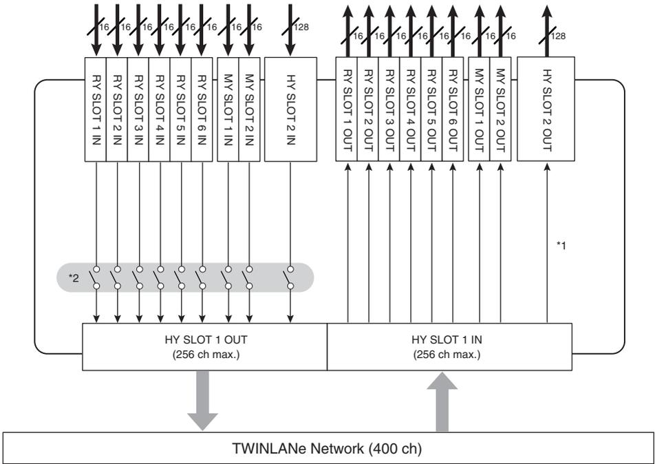
\*1) In mode 2, you can patch signals from the DSP engine to the HY SLOT 2 output via the TWINLANE network.
