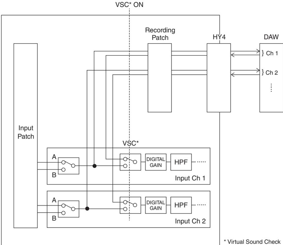
\* Each channel can individually be set to ON/OFF when switching to virtual sound check. This allows a virtual sound check that mixes playback from the recorder with actual stage inputs.
