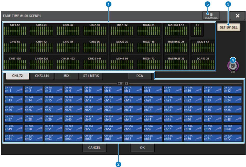
In this popup window you can select the channels to which Fade will be applied, and adjust the fade time.
