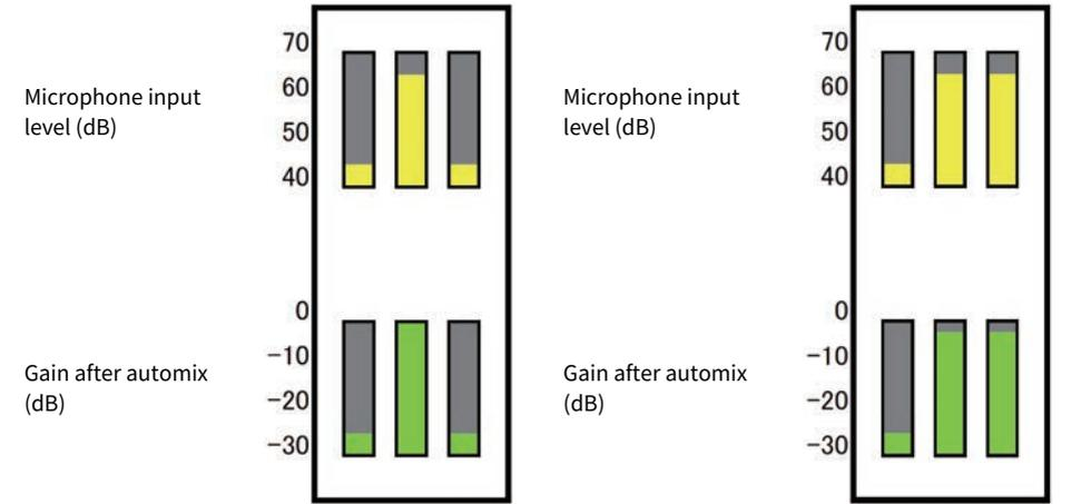
If one person speaks, that microphone's gain level will fade up instantly, while the other microphone gains will be reduced. If a different person speaks, the same effect will be obtained.
