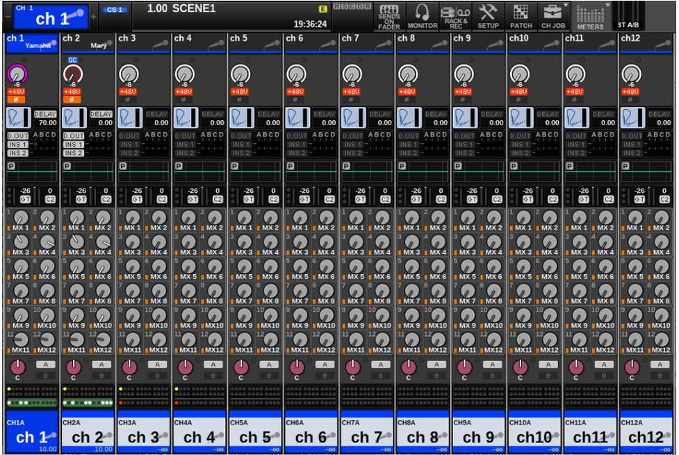
The actor library name has been added as an indicator for the channel name area. (Pressing the [SHIFT] key will display the CUE status, as with normal mode.) When the EQ or dynamics parameters have been changed, an asterisk will appear in the actor library name.
