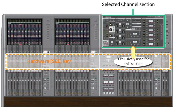
A [SEL] key is used to select the corresponding channel for the Selected Channel section (hardware). However, the [SEL] keys can also be linked to on-screen selected channels to assign channels to a DCA or mute group.
