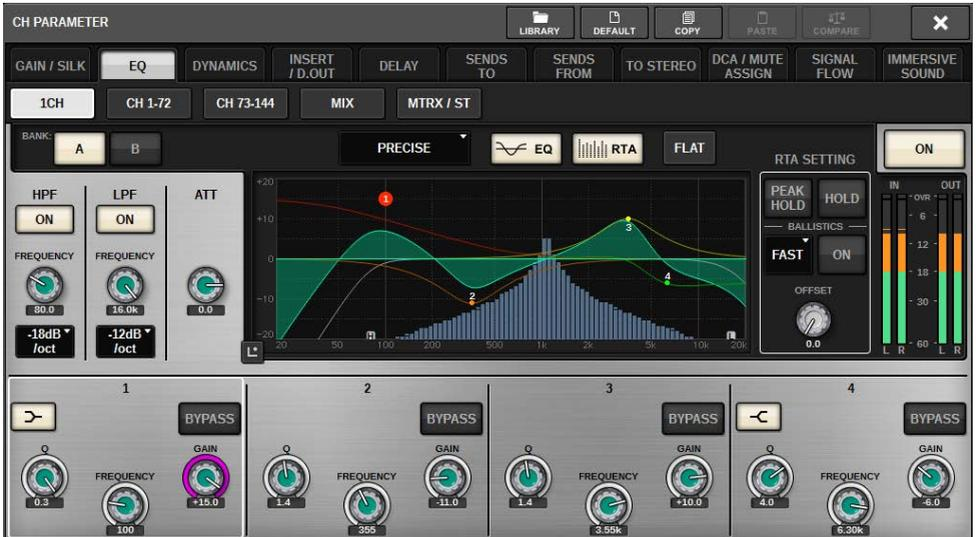
You can switch between popup windows using tabs as needed. Some popup windows show several buttons called “tool buttons” at the top of the window. You can use these tool buttons to recall libraries or to perform copy and paste operations. Press the “x” symbol located in the upper right corner to close the popup window and return to the previous screen.
