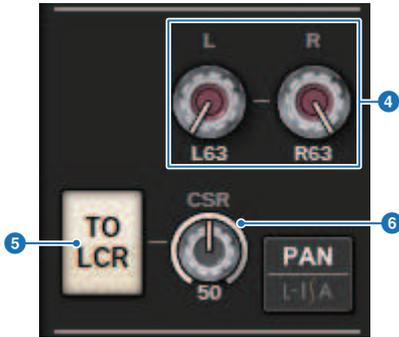
In the TO STEREO popup window, if the PAN/BALANCE select button is set to PAN, the L and R PAN knobs **4** are shown, enabling you to specify the panning of the signal. If you use the ST/LCR mode select button to select LCR, the LCR button **5** and CSR knob **6** appear. The LCR button turns on/off the signal that is sent from the channel to the STEREO bus, and the CSR knob specifies the level ratio between the signal that is sent to the STEREO A (L/R) bus and to the STEREO B (C) bus.
