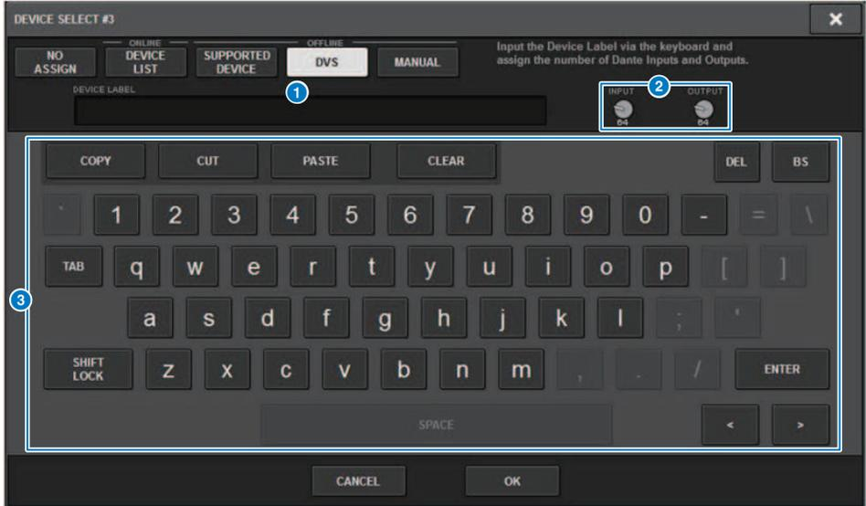
Here you can enter a device label for an I/O rack, and mount it offline.
