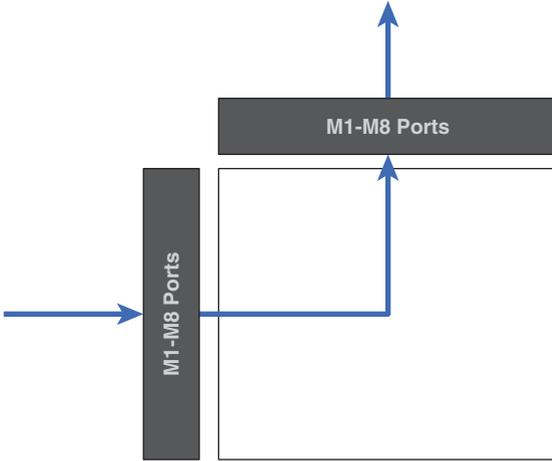
Between slots, patching can be done via SLOT BRIDGE patch (36 outputs and 36 inputs for each slot).
