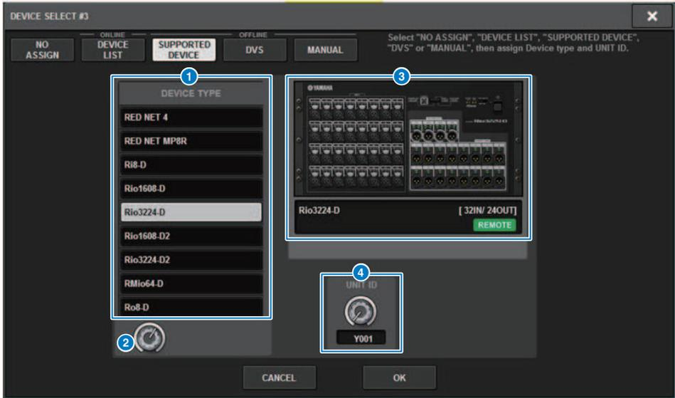
Here you can select from the supported I/O racks, and mount a device offline.
