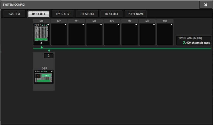
Press an I/O rack select button (in this case the M1 button). The I/O rack settings popup window will appear.
