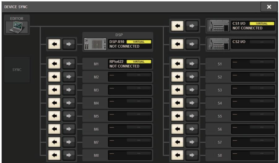
When connecting PM Editor, you must specify the data sync direction for the DSP engine.
