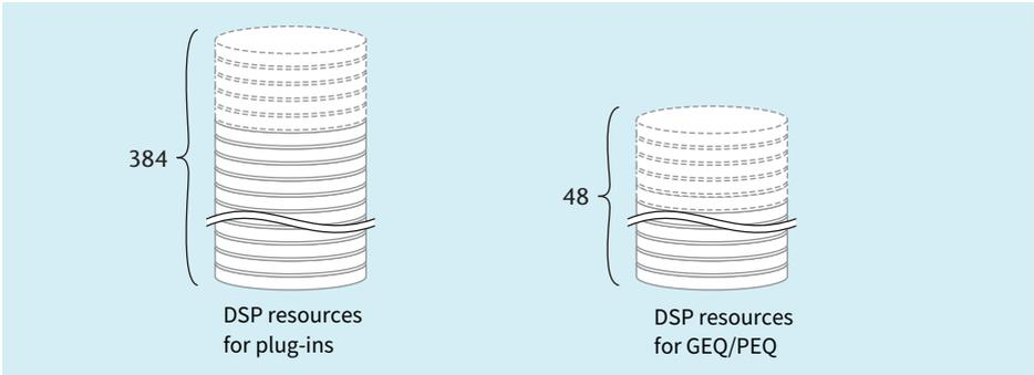
Plug-ins and GEQ/PEQ each feature their dedicated DSP resources. DSP resources are consumed each time a plug-in is mounted or a GEQ/PEQ is inserted. DSP resources usable by plug-ins are divided into 384 units, and the DSP resources that are usable by GEQ/PEQ are divided into 48 units. For details on the DSP resources used by each plug-in or GEQ/PEQ, refer to the data list.
