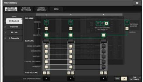
For more information on the settings, refer to the “SURFACE SETTINGS1” (p.851) of the Preferences Settings. The selected layer will be indicated by a bold white frame in the meter area. Also, the layer of the linked bay will be indicated by a thin white frame.
