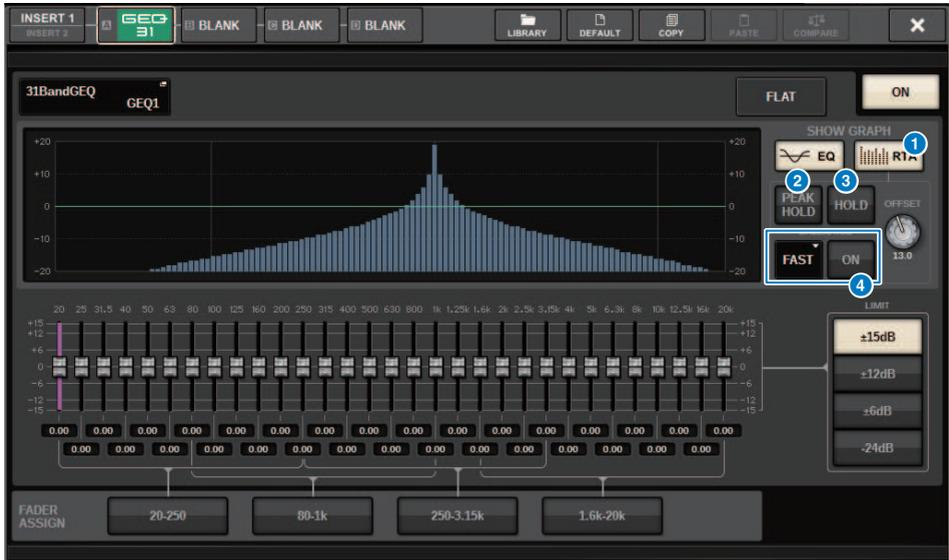
Press the rack container of the rack (which contains an inserted GEQ) to open the GEQ popup window.
