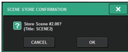
If Overlay is enabled and the STORE WITH OVERLAY APPLIED button is turned on, a dialog box will appear.
