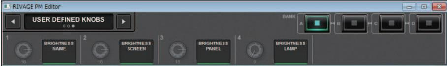
You can switch the function assigned in the USER DEFINED KNOBS screen on or off. Buttons for the functions that you cannot control in PM Editor will be grayed out.
