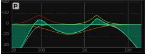
This field indicates the approximate response of the EQ. Press this field to open the HPF/EQ (1CH) popup window, in which you can set the HPF, LPF and EQ. This field will be grayed out on channels for which the EQ is disabled.
