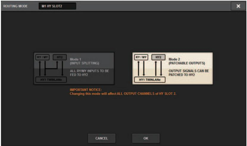
This window enables you to switch the routing mode for HY slot 2.
