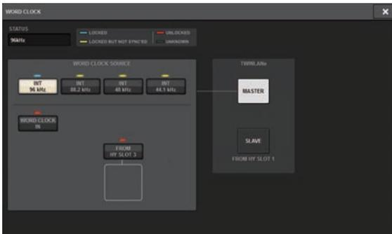
The default value is 96kHz. If the unit is operating correctly with the selected clock, the indicator for the selected clock will light blue, and the clock frequency will be displayed in the upper left of the MASTER CLOCK SELECT field.
