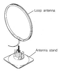
⑤ Tune to an AM station and then position the loop antenna for best reception. Orient the AM loop antenna so that the best reception is obtained. Try other stations, and find the position that gives the best overall reception.
