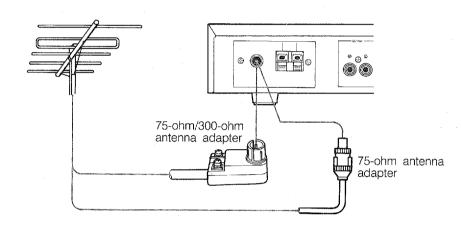
\* When using a 75-ohm/300-ohm antenna adapter (separate purchase), follow the instructions shown below.
