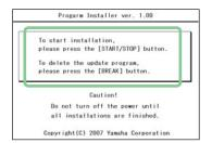
**Press the [START/STOP] button to start installation.** Go on to **step 4**. (Executing the installation).
