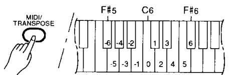
This function allows the MIDI note data transmitted by the Clavinova to be transposed up or down in semitone increments by up to plus or minus 6 semitones. The pitch of the Clavinova itself is not affected.
