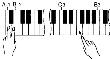
**1** To tune up (raise pitch), hold the **A-1** and **B-1** keys simultaneously.
