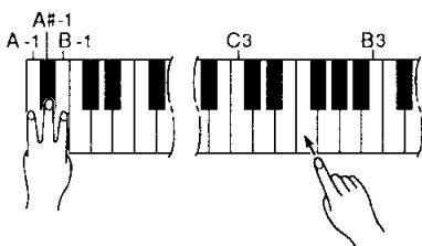
**1** To restore standard pitch ( $A3 = 440$  Hz), hold the **A-1**, **A#-1** and **B-1** keys simultaneously.
