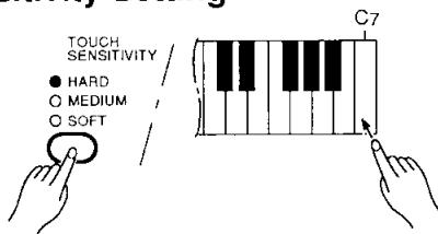
Press the C7 key while holding the [TOUCH SENSITIVITY] button to memorize the current touch sensitivity setting. The memorized setting will be retained in memory for about one week after the power is turned off, then the default setting will be restored. To keep the memorized setting for longer periods, turn the power on briefly at least once a week.
