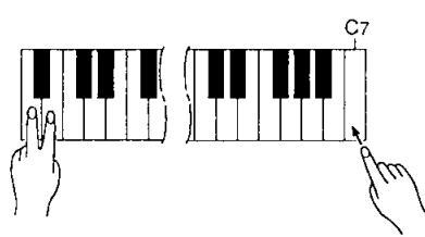
\* Standard pitch ( $A3 = 440$  Hz) is set when the [POWER] switch is initially turned ON. The power-on pitch setting can be changed, however, by pressing the **C7** key while still holding the **A-1/B-1**, **A-1/A#-1**, or **A-1/A#-1/B-1** key combinations after setting the desired pitch.
