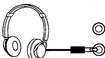
Two pairs of standard pair of stereo headphones can be plugged in here for private practice or late-night playing. The internal speaker system is automatically shut off when a pair of headphones is plugged into either of the HEADPHONES jacks.
