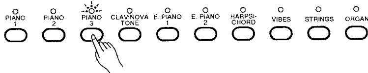
The 10 demo tunes are selected via the voice selectors. Press a selector to start playback of the corresponding tune, featuring the voice normally selected by that voice selector button. The demo tunes will play in sequence until stopped, starting with the selected tune. The voice selector indicator will flash during demo playback.
