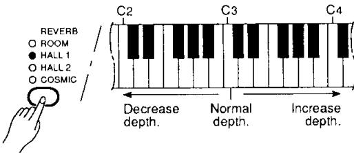
The depth of the selected reverb effect can be adjusted for the current voice by using the C2 through C4 keys on the keyboard while holding the [REVERB] button. The C3 key sets the "normal" depth for the selected effect. Keys to the left of C3 decrease the reverb depth, while keys to the right of the C3 key increase the reverb depth. Separate reverb settings can be made for each effect and voice.
