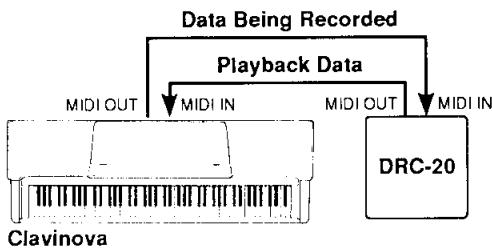
This same type of musical information transfer is used for MIDI sequence recording. A sequence recorder such as the Yamaha DRC-20 Disk Recorder can be used to “record” MIDI data received from a Clavinova, for example. When the recorded data is played back, the Clavinova automatically “plays” the recorded performance in precise detail.
