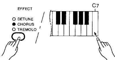
The CLP-134 allows different effects to be set for each voice so that the appropriate effect is automatically recalled whenever a voice is selected.
