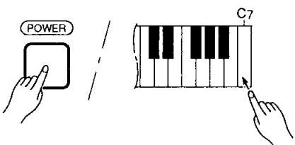
All dual mode, reverb, effect, touch sensitivity, pitch control, and individual key tune settings can be restored to their original factory preset (default) values by holding the C7 key while turning the [POWER] switch ON.
