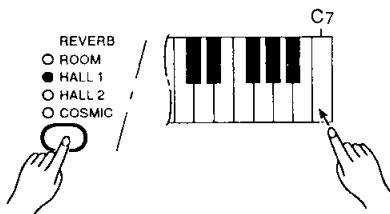
Press the C7 key while holding the [REVERB] button to memorize the current effect type and all depth settings made since the power was turned on. The memorized settings will be retained in memory for about one week after the power is turned off, then the default settings will be restored. To keep the memorized settings for longer periods, turn the power on briefly at least once a week.
