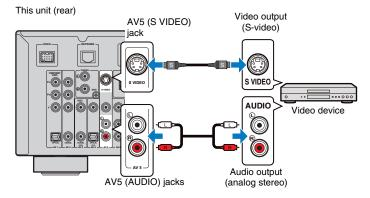
If you select the input source by pressing AV5, the video/audio played back on the video device will be output from this unit.
