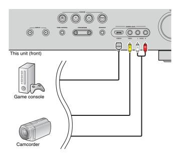
If you select "V-AUX" as the input source by pressing V-AUX, the video/audio played back on the device will be output from this unit.
