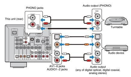
If you select the input source by pressing AV1~6, AUDIO1~2 or PHONO, the audio played back on the audio device will be output from this unit.
