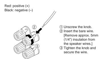
\* Banana Plug connections are also possible (except for U.K. and Europe models). Simply insert the Banana Plug connector into the corresponding terminal.
