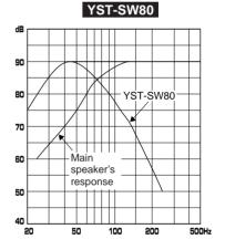
When combined with an 8" or 10" acoustic suspension, 2 way system
