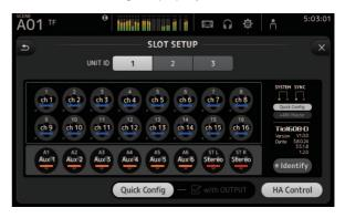
To assign the Tio1608-D inputs to the TF series mixing console, set the input select on the console's INPUT screen to "SLOT".
