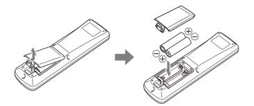
A diagram inside the battery compartment shows which way the batteries should be installed. Make sure you insert them correctly.
