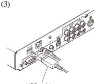
USB cable Cable USB Kaбeль USB USB电缆 USB電纜 USB 케이블 Connect the USB cable extending from the drive to the USB port on the rear panel of the control unit.
