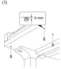
Insert the three restraining screws  $(5 \times 12)$  into the marked nuts underneath the bass side key bed, then tighten the screws, leaving a gap of about 5 mm between head of the screw and piano body.
