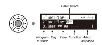
Confirm that the cursor is on the timer switch, then press [+/YES] and [–/NO] to switch the timer play on and off.
