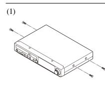
Remove the four screws from the sides of the control unit.
