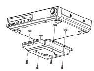
Attach the drive and case assembly to the bottom of the control unit, using the four screws  $(3 \times 6)$  supplied with the Disklavier.
