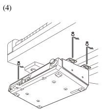
Fit the "slots" of the metal suspension bracket containing the control unit to the screws mentioned in step (3).
