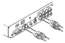
Connect the cables extending from the piano to the appropriate connectors/jacks on the rear panel of the control unit.
