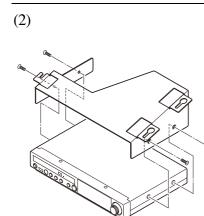
Place the metal suspension bracket, supplied with the Disklavier grand model, over the control unit, then secure the metal suspension bracket to the control unit using the four screws  $(4 \times 10)$  supplied with the Disklavier.
