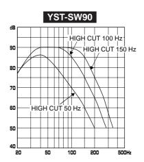
The figures below show the optimum adjustment of each control and the frequency characteristics when this unit is combined with a typical main speaker system.
