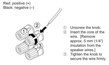
\* Banana Plug connections are also possible (except for U.K. and Europe models). Simply insert the Banana Plug connector into the corresponding terminal.
