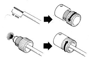
In connecting the R and L speaker cords, observe the "+" and "-" markings. If the "+" and "-" cords are reversed, the sound will be unnatural and will lack bass. Speaker cords should be cut as short as possible; do not coil up excess cord on the floor. Also, do not bundle with cords from other system components.
