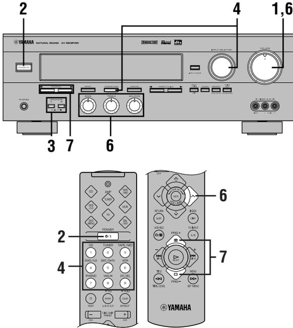
**4** Select the desired input source with **INPUT SELECTOR** (or the input selector buttons). (Turn on the TV monitor for video sources.)
