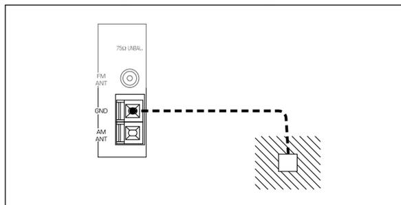
For maximum safety and minimum interference, connect the antenna GND terminal to a good earth ground. A good earth ground is a metal stake driven into moist earth.
