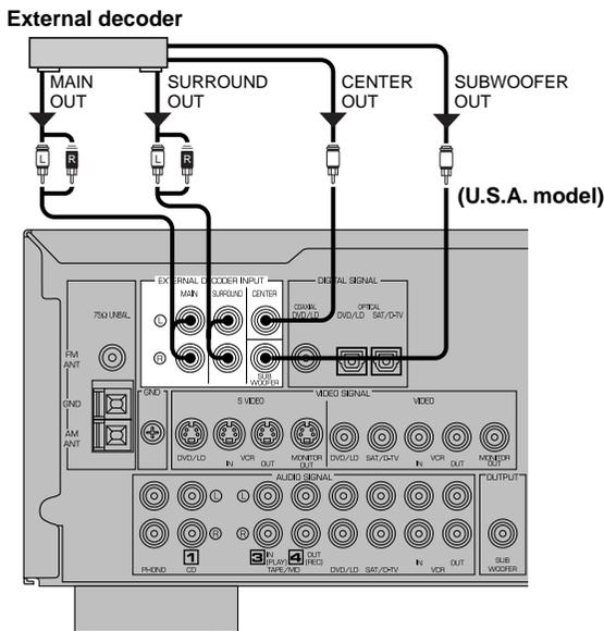
This unit has additional 6-channel audio signal input terminals for connecting an external decoder to this unit. Connect the 6-channel audio signal output terminals of the decoder to the EXTERNAL DECODER INPUT terminals of this unit.
