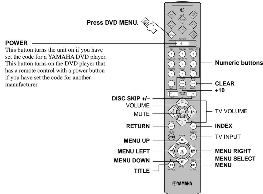
The dark-shaded buttons do not function. Refer to the instructions for details of each component.
