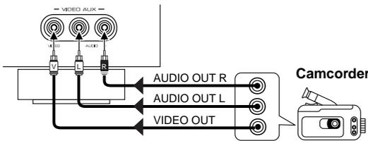
These terminals are used to connect any video input source such as a camcorder to this unit.
