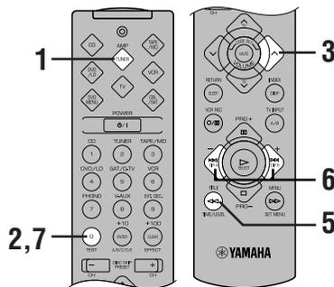
**1** Press AMP(TUNER) on the component selector.
