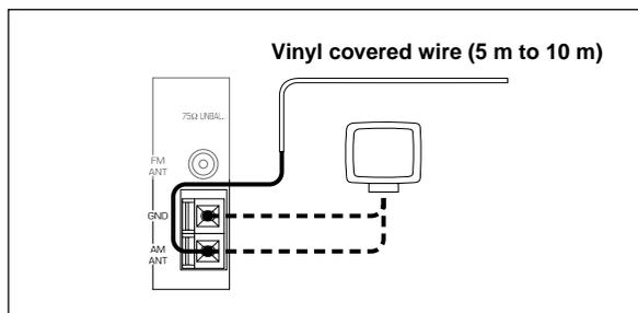
If you cannot obtain good reception with the AM loop antenna, connect 5 m to 10 m of vinyl covered wire to the AM ANT terminal and extend it outdoors from a window.
