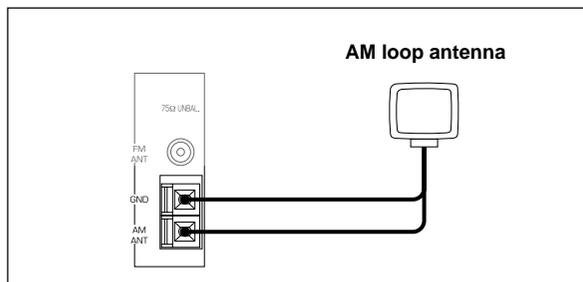
The AM loop antenna can be removed from the stand and attached to a wall, etc. However, note that the reception sensitivity may deteriorate if the antenna is attached to a metal or steel reinforced wall.
