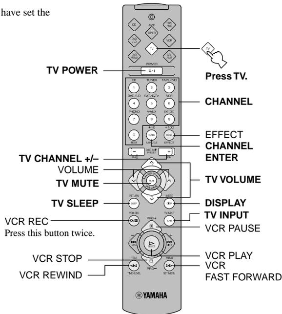
The dark-shaded buttons do not function. Refer to the instructions for details of each component.
