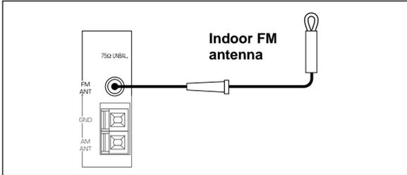
Firmly insert the connector into the FM ANT terminal. The indoor FM antenna is only a simple antenna. For reception with better sound quality, installing the outdoor FM antenna (commercially available) is recommended.
