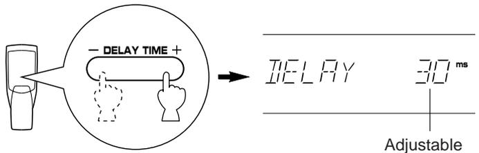
\* When the **DELAY TIME** key is pressed, sound is momentarily interrupted.
