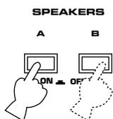
\* If you use two main speaker systems, press both the A and B switches.
