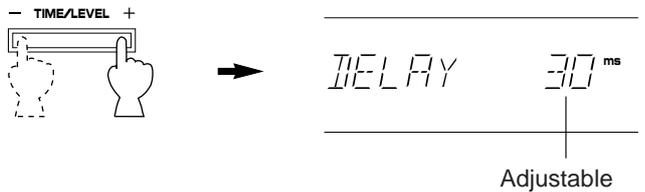
\* When the **TIME/LEVEL** button is pressed, sound is momentarily interrupted.
