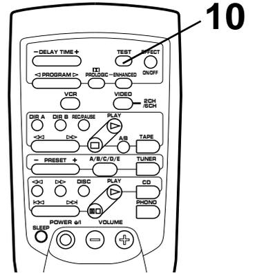
**9** Adjust the sound output levels of the center speaker and the rear speakers so that they become almost as same as that of the main speakers.
