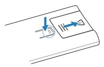
2 Insert an object such as a fine-tip ballpoint pen in the way shown by the arrow and remove the battery.
