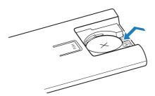
3 Insert a new battery and slide the cover back into its position in the direction of the arrow.
