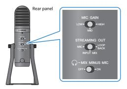
Once you've made the settings on this product, launch the "AG Controller" app and click "Sound Check" at the bottom of the screen. Adjust the volume to check the sound on the Sound Check screen that appears.
