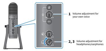
3 While speaking into the mic with the [□] mark facing straight toward you, adjust the headphone/earphone volume. Adjusting the volume for the headphones or earphones has no effect on the volume of the livestreaming audio.
