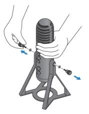
Attaching this product onto a mic stand or desk-mounted microphone boom arm > How to attach
