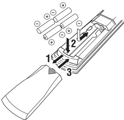
**1** Press the ▼ part and slide the battery compartment cover off.
