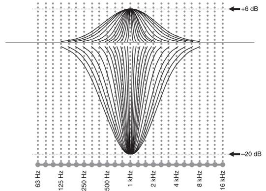
YPAO adjusts frequency characteristics to suit your listening requirements using a combination of the above three parameters (Frequency, Gain and Q factor) for each equalizer band in this unit's parametric equalizer. This unit has 7 equalizer bands for each channel.
