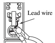
**4** Insert the cable wire into the slot, and clamp it with pliers.
