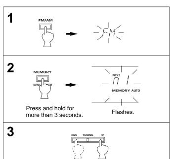
To tune to higher frequencies, press right side once. To tune to lower frequencies, press left side once.
