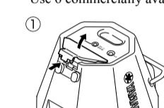
To remove the battery cover, push the tab while lifting the cover upward.
