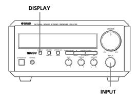
Press and hold **DISPLAY** for about two seconds so that "Dimmer  $\pm 0$ " appears on the display. While holding **DISPLAY**, turn **INPUT** clockwise to increase or counterclockwise to decrease brightness.
