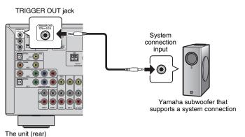
• You can configure the trigger function settings in "Trigger Output" (p.95) in the "Setup" menu.
