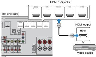
If you select the input source by pressing HDMI 1–5, the video/audio played back on the video device will be output from the unit.
