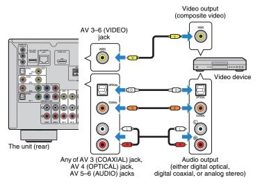
If you select the input source by pressing AV 3–6, the video/audio played back on the video device will be output from the unit.
