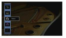
3 Use the cursor keys  $(\triangleleft/\triangleright)$  to select an input source to be configured and press the cursor key  $(\triangle)$ .
