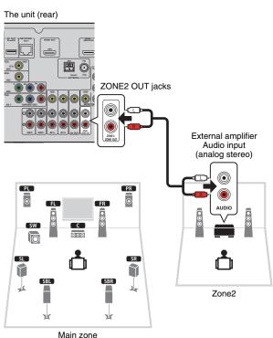
When Zone2 output is enabled (p.70), the surround back speakers in the main zone do not output sound.
