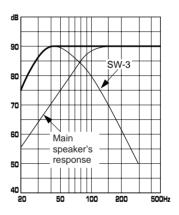
• When combined with a 6" or 8" acoustic suspension, 2 way system
