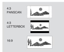
Select the aspect ratio of the TV to be connected. **4:3 PANSCAN**  $\rightarrow$  when you connect a normal TV to the DVD player. Displays the wide picture on the whole TV screen with a portion automatically cut off.
