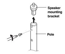
**4** Attach the speaker mounting bracket to the speaker by screwing it into the screw hole on the bottom of the speaker.
