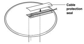
The setup has completed. In the same way, set up the other stand.
