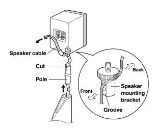
**6** Pull out the speaker cable in the length of 15 to 16 cm from the speaker mounting bracket. Then attach the speaker mounting bracket to the pole so that the speaker cable fits to the cut in the pole. This will lock the speaker cable. After that, fasten the screw.
