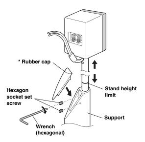
\* The inside of the rubber cap has a space for storing the wrench after the setup.
