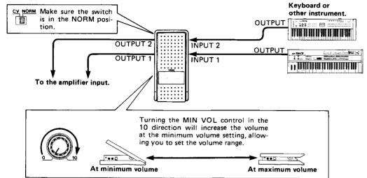
Signals fed into INPUT 1 are output through OUTPUT 1; INPUT 2 is output through OUTPUT 2. Connections are made with standard phone plugs.
