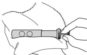
4. Return the piston to its corresponding valve casing.
