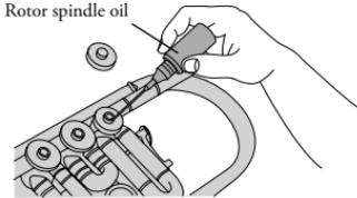
2. Apply some rotor spindle oil to point where the rotor rotates. Replace the rotary valve cap and move the lever a few times to distribute the oil evenly.
