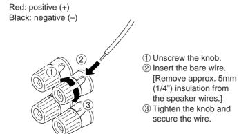
\* Banana Plug connections are also possible (except for U.K. and Europe models). Simply insert the Banana Plug connector into the corresponding terminal.
