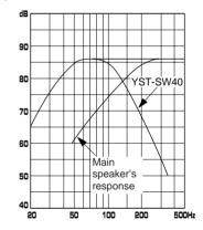
When combined with 5" acoustic suspension, 2 way system
