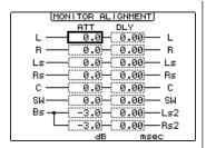
parameters can be set  $-\infty$ , -12 dB to +12 dB in 0.1 dB steps. The Delay parameters can be set from 0 to 30 msec in 0.02 msec steps.
