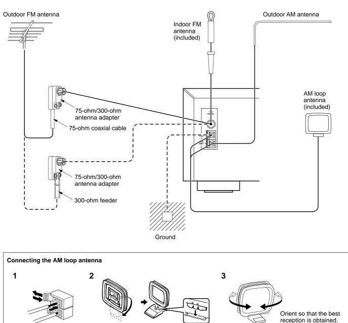
\* The AM loop antenna should be placed apart from the main unit. The antenna may be hung on a wall.
