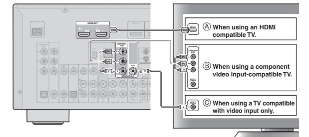
Video input to this unit is output to a TV using output jacks of the same kind.
