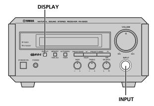
Press and hold **DISPLAY** for about two seconds so that "Dimmer ±0" appears on the display. While holding **DISPLAY**, turn **INPUT** clockwise to increase or counterclockwise to decrease brightness.
