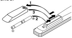
Remove the battery compartment cover.
